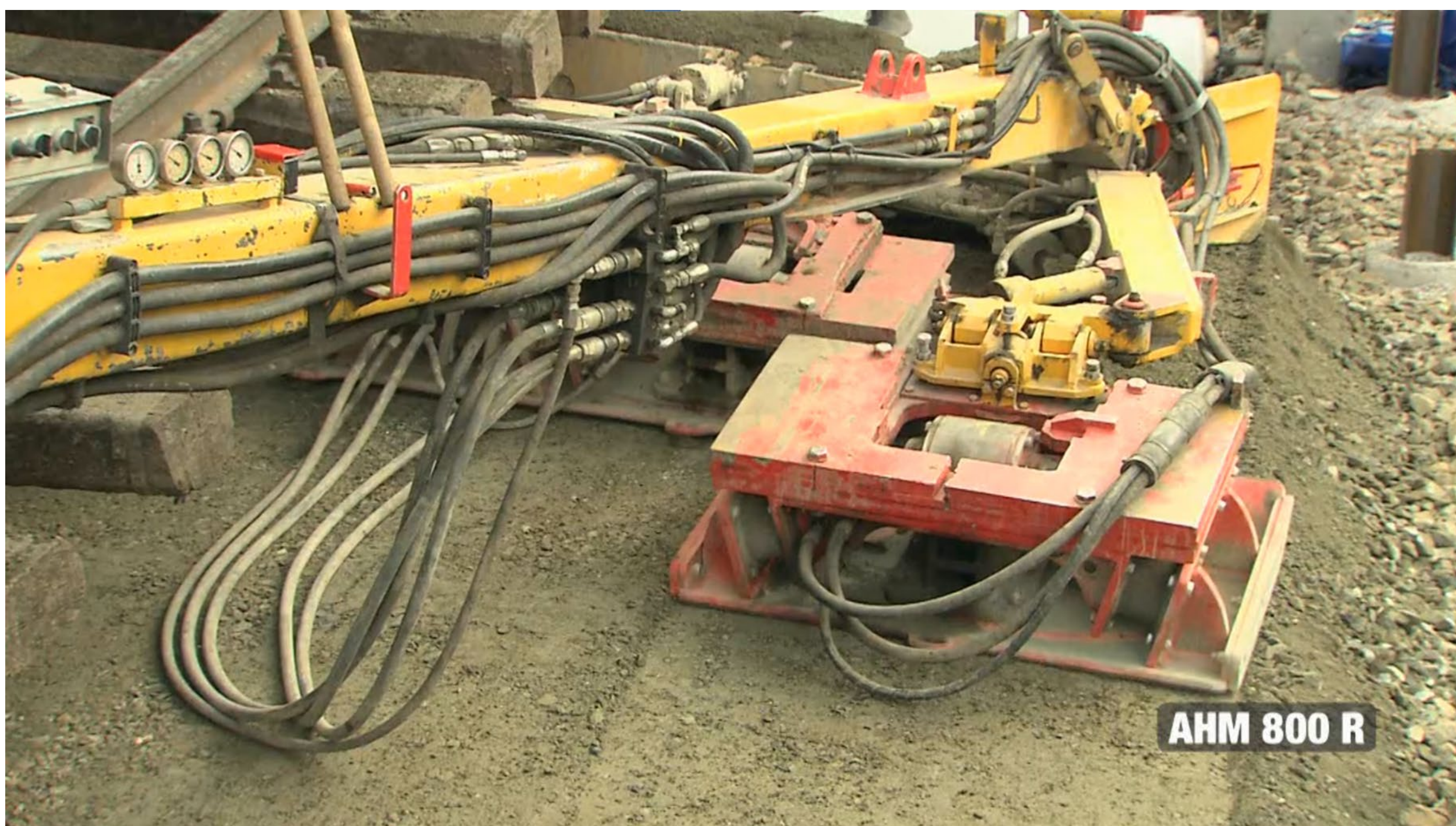
Figure 1. Plate compactors during substructure rehabilitation
