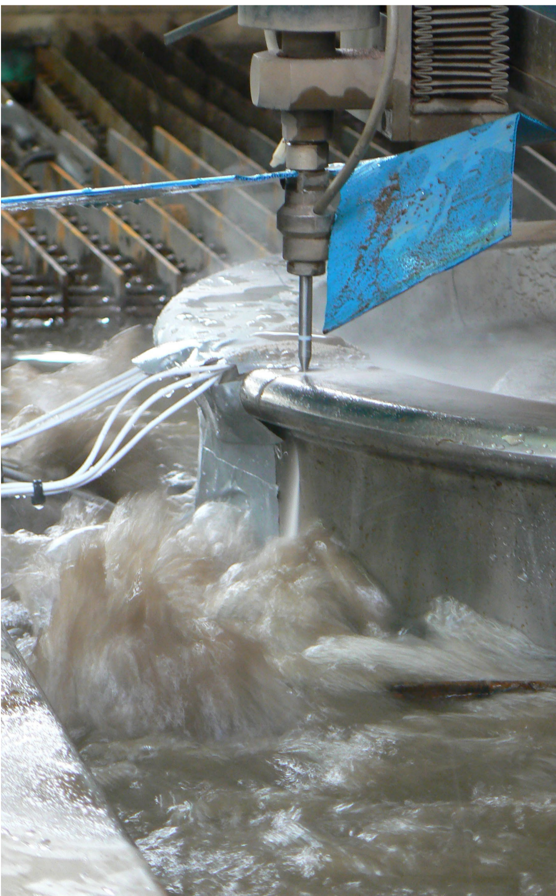
Figure 3. Waterjet cutting of wheel rim
