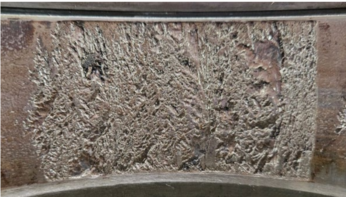
Figure 3: Cup Damage, Bearing R7
