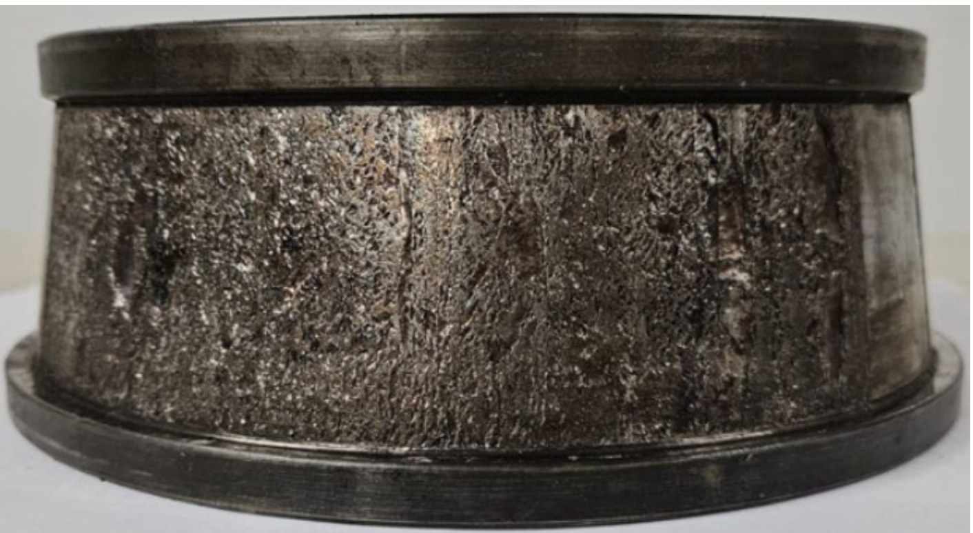
Figure 4: Cone Damage, Bearing R7
