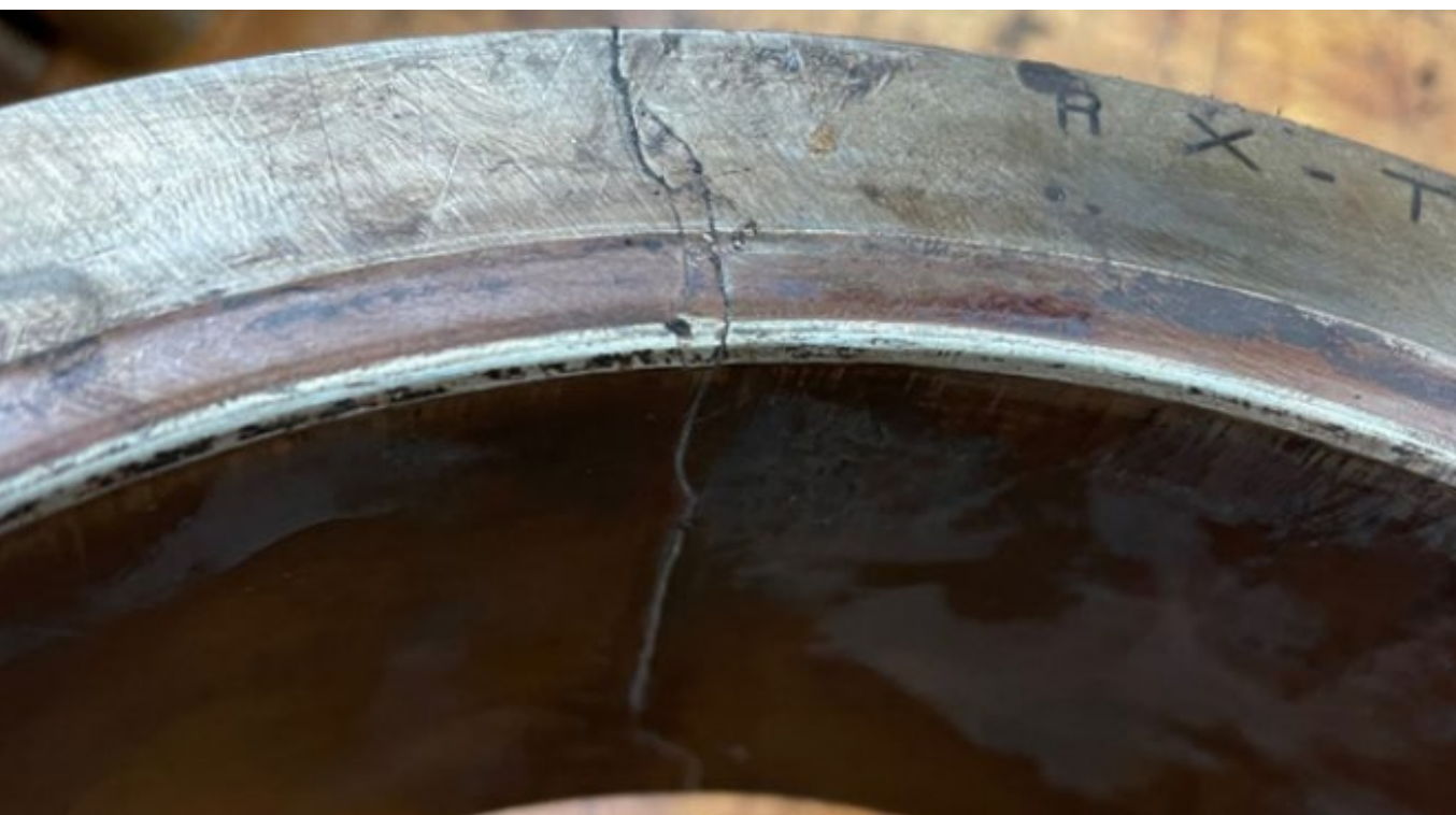
Figure 5: Cracked Cone, Bearing R7
