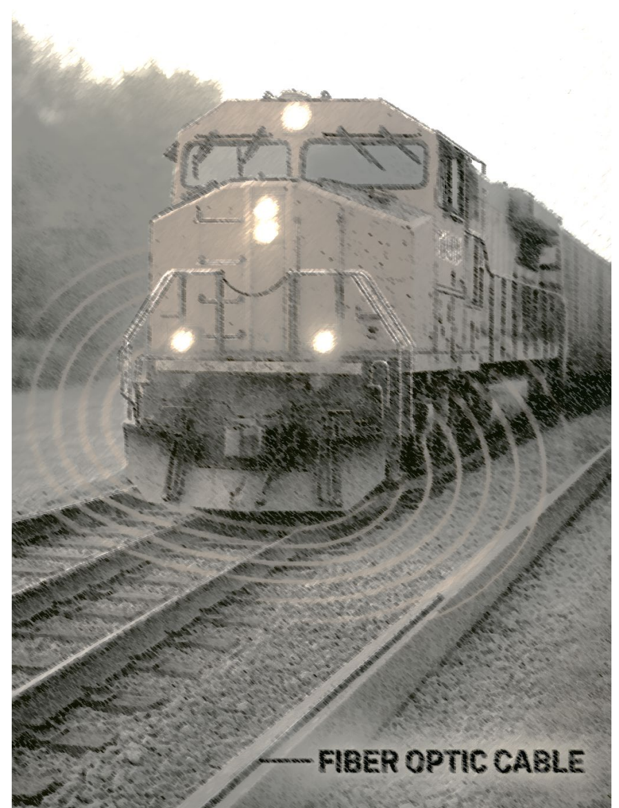
Figure 1. Train-induced vibrations along the sensor.
