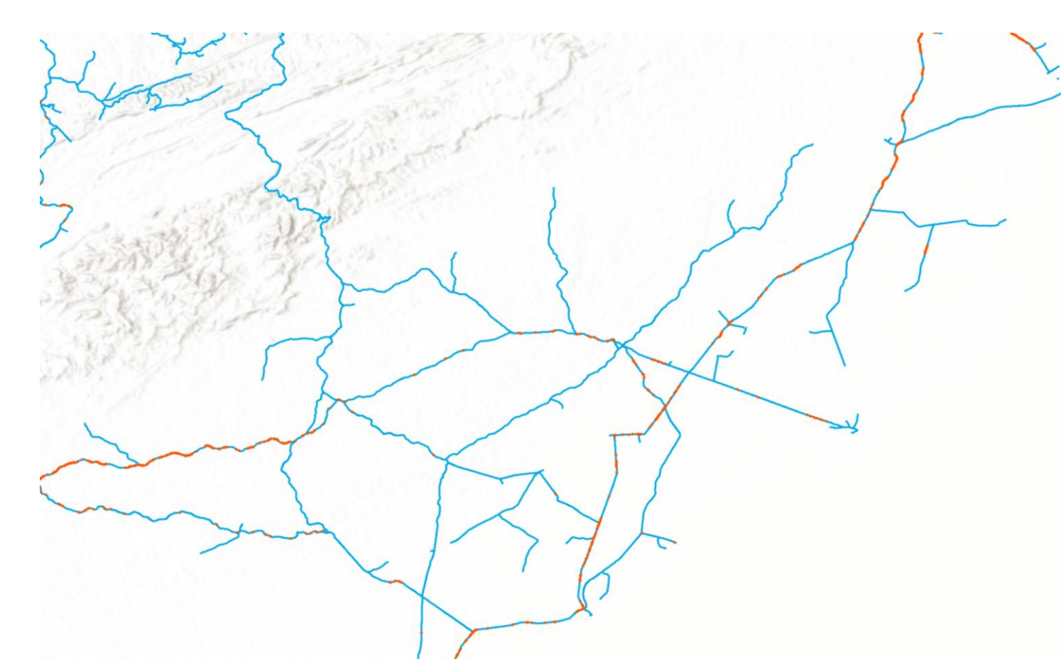
Figure 4. Predicted Top 10% Risk of Broken Rails over Studied Railroad Network
